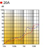
Common mode / Asymmetric (L-G) \_\_\_\_\_\_ Differential mode / Symmetric (L-L) \_\_\_\_\_
